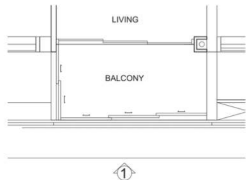
23RD TO 33RD STOREY (APPLICABLE TO ALL TYPES EXCEPT TYPE A1 AND A2) , 35TH TO 43RD STOREY (APPLICABLE TO ALL TYPES EXCEPT TYPE A1 AND A2) AND #44-03: TYPICAL RETRACTABLE BALCONY SCREEN (CLOSED) - PLAN
